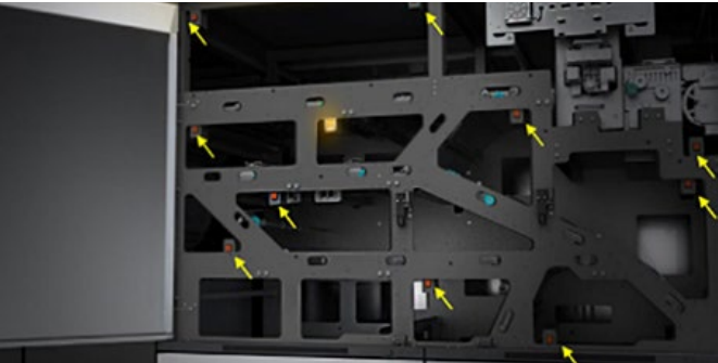
Navigation LED LED lights guide the operator to areas of the press that need attention.
